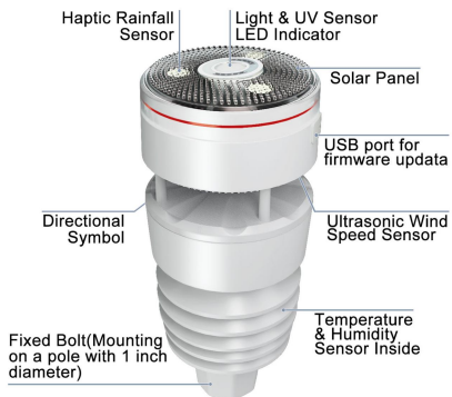
Figure 3 Sensor package assembly components
